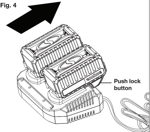
**CAUTION!** FIRE HAZARD. When removing the batteries from the charger, be sure to unplug the charger from the outlet first, then remove the batteries from the charger.
