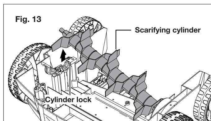
4. Insert the raking cylinder and press it into the holder. Refasten the lock and fix the assembly with the lock screw (Fig. 14).
