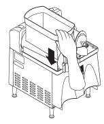
5. Slide into place and push down until the hopper lock plunger(s) snap into place.
