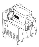
**4.** Thoroughly rinse the hopper(s) and install over the auger(s) and cooling drum(s).
