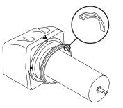
Install each hopper seal over 8. the flange at the rear of the cooling drums as shown.
