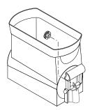
**3.** Install auger nose bushing into inside front of hopper.
