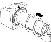
2. Align the auger shaft(s) with the auger(s). Push the auger(s) as far as they will go and rotate so the flat face of the auger shaft is aligned with the flat face of the auger nose.
