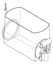
**13.** For models with PAF, install level probes into slots at top rear of PAF hoppers.
