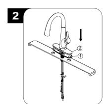
Optional Deck Plate Installation: Before installation, align the hole in the gasket (1) and deck plate (2) with the mounting hole in the sink. Place the faucet assembly through the deck plate (2) and mounting hole in the sink until the faucet assembly sets on top of deck plate (2).
