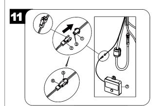
Install the sensor cable (1) to the connection (2) of the timer (7). Ensure the holes (3) on the sensor cable (1) and the pins (4) on the timer (7) are aligned to one another to ensure proper installation. Ensure they are tightly connected by firmly pushing together. If it is necessary to remove the timer (7), squeeze the tabs (5 & 6) on the sensor cable (1) and timer (7) at the same time.
