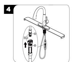
Push the quick connector (2) with the blue tab firmly upward and attach it to the receiving block (1) with blue. Pull down moderately to ensure the connection has been made. If it is necessary to remove the quick connector (2), squeeze the tabs on the quick connector (2) and then pull down to disconnect.
