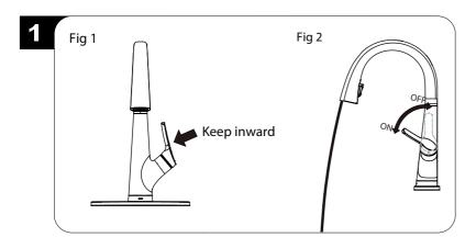
Make sure the the faucet is closed and do not open the handle outward, as shown in the Fig 1. Maintain the state of the Fig 1, pulling the handletowards yourself will activate the filtered water, as shown in the Fig 2.
