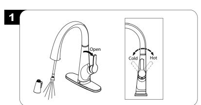
Pull the hose assembly out of the spout and remove the spray head by unscrewing it from the hose in a counterclockwise direction. Be sure to hold the end of the hose down into the sink and turn the faucet to the warm position where it mixes hot and cold water.
