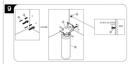
Before installation, select the location for the filtration manifold (5). The screws should be placed a minimum of 15 in. above the bottom of the floor where the filtration system is to be mounted. Any distance lower than 15 in. may result in the filter set (6) interfering with the floor when removing the filters for maintenance.
