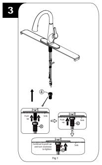
From underneath the sink, secure the faucet assembly to the sink with the FastMount™ system (4). Push the FastMount™ system (4) up over the threads until it stops against the bottom of the sink, then hand turn (clockwise) to tighten (Fig 1).
