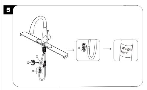
Install the weight clip (2) at the point of the hose marking "weight here". Insert the weight (1) onto the clip (2) by sliding it down onto the clip (2).
