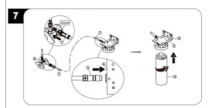
Connect the end of the hose (7) with the quick connector to the tee connector (6). Push the quick connector with the green tab on the hose (7) firmly upward and attach it to the receiving block with green on the tee connector (6). Pull moderately to ensure the connection has been made. If it is necessary to remove the quick connector, squeeze the tabs on the quick connector and then pull to disconnect.
