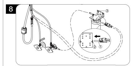
Connect the end (1) with outlet indicated by the tag of the outlet hose into the end (2) with outlet indicated of the filtration manifold (3). Pull moderately to ensure the connection has been made.
