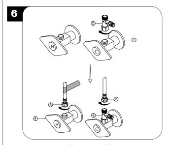
Attach the tee connector (5) onto the outlet of the cold water supply valve (1) and tighten with wrench. Do not overtighten. Thread the nut (2) on the cold supply line onto the tee connector (5) and tighten with wrench. Do not overtighten. Thread the nut (3) on the hot supply line onto the outlet of the hot water supply valve (4) and tighten with wrench. Do not overtighten.
