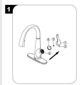
Shut off water supply. With valves in "closed" position, loosen the set screw (2) from handle (1) and remove handle (1) from faucet. Loosen the screw (3) and unscrew the cap (4) from the cartridge nut (5).
