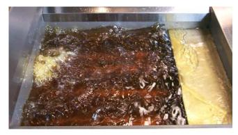
Allow the oil to bubble for 10-15 seconds to ensure evacuation of all oil in the return lines.
