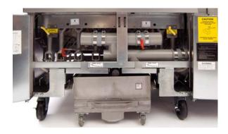
The filter pan slides under the fryer (left), connecting with a male connector (right). Ensure that the pickup tube is securely coupled with this connector. Its location may vary based on model.
