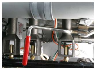
After filtering is complete, close the red drain handle to start refilling the frypot.
