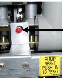
**Filter Pump Reset Switch**
