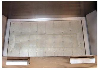
Support grid properly placed in filter pan.
