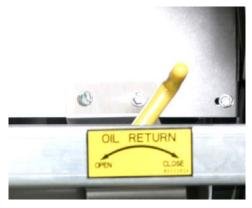
Turn the yellow handle to open the oil return valve and activate the filter pump.
