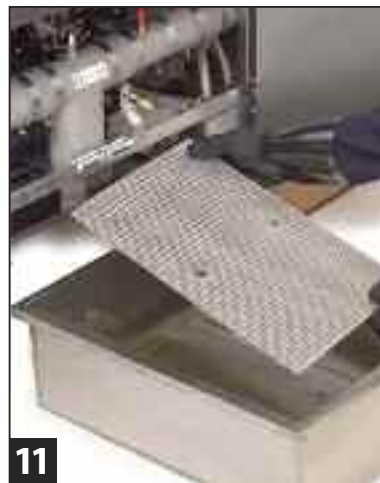
11 Remove and wipe off filter screen with paper towels.
