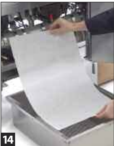
14 Install filter paper making sure it evenly laps all pan walls.
