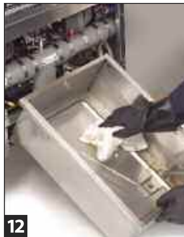
12 Wipe out filter pan with paper towels.
