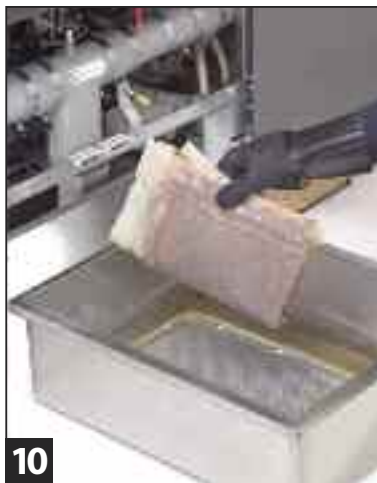
10 Remove and discard used filter paper.
