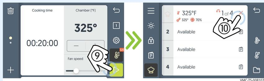
At the end of the cooking process, the oven sounds an alert and the chamber light and door handle light flashes. The cooking done screen displays.
