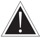
Used to indicate the presence of a hazard that can or will cause minor or moderate personal injury or property damage if the warning included with this symbol is ignored.
