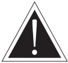
Used to indicate the presence of a hazard that **WILL** cause severe personal injury, death, or substantial property damage if the warning included with this symbol is ignored.
