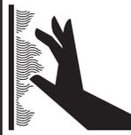
METAL PARTS OF THIS EQUIPMENT BECOME EXTREMELY HOT WHEN IN OPERATION. TO AVOID BURNS, ALWAYS USE HAND PROTECTION WHEN OPERATING THIS APPLIANCE.
