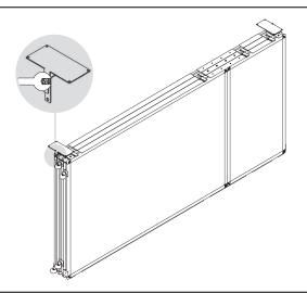
Attach wall mount hinges using bolts attached to wall mount bracket.
