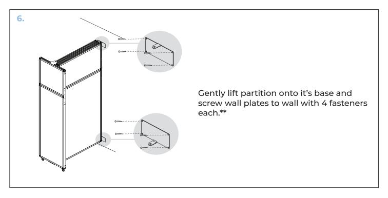
\*\*Due to differing wall types fasteners are not included with wall plates. Please evaluate wall material and consult local hardware professional before installing wall plates to wall for a secure installation.
